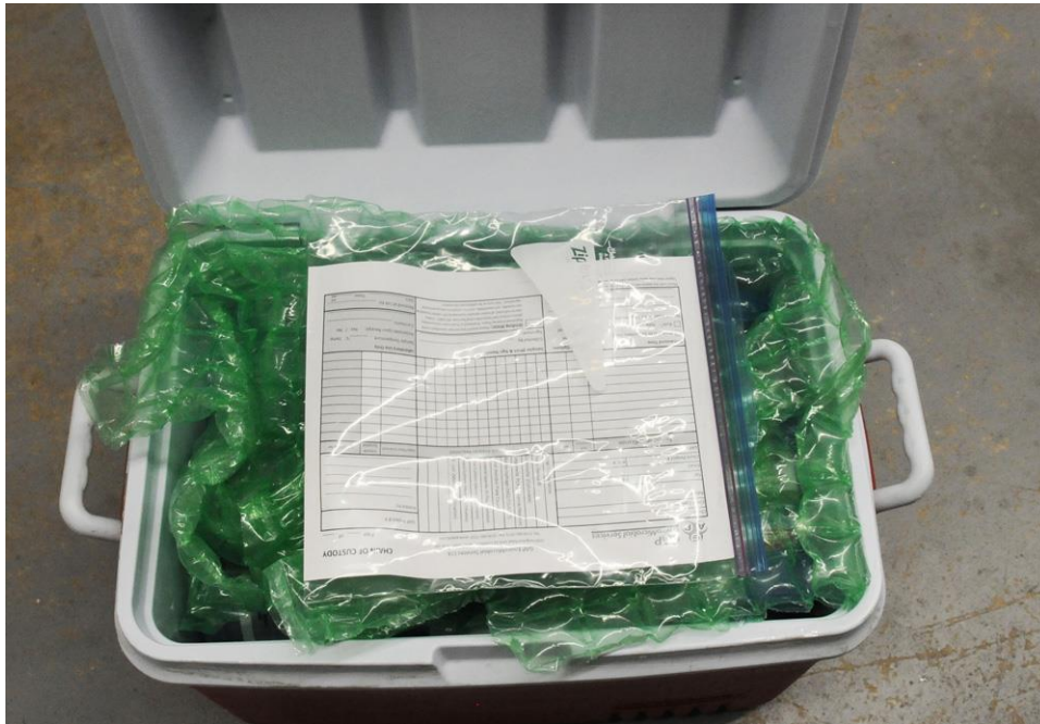
Figure 4. Packing material (with Chain of Custody) added to the cooler to fill any voids inside the cooler.
